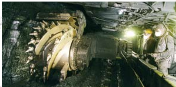
Face Support with cutting rollers.
