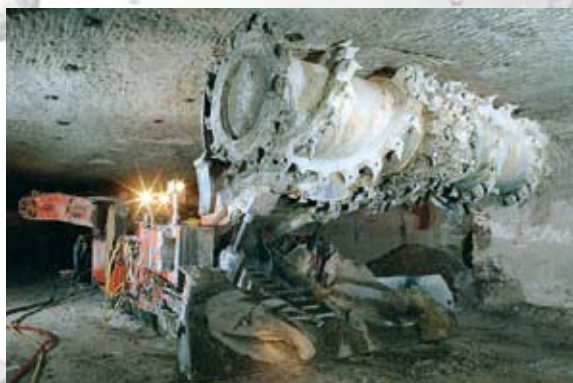
Room-and-pillar support using Continuous Miner.
