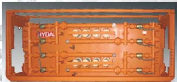
High Pressure Filter panel for filtration of the longwall hydraulics or the sprinkling water.
