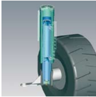
Cylinder for the suspension system on load haul dumpers.
