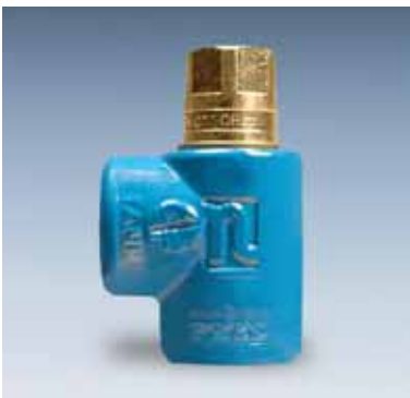
TBDE 201 Relief valves, 3/4" BSP ported, for flows from 20 l/min up to 160 l/min at max. 300 bar, depending on pressure setting. Adjustable and sealed.
