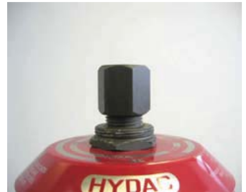
Gas side of the accumulator shown with sealing cap
