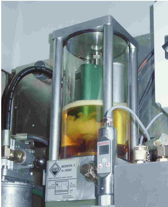
*REDFOX C-Ty, a complete turnkey equipment with monitoring, degassing and filtration functions.*
