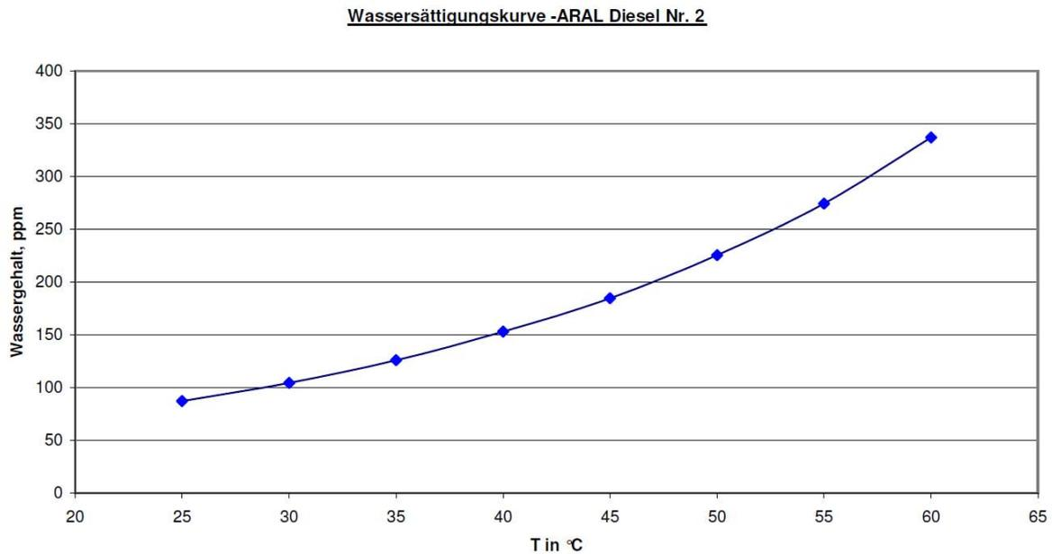
Figure 1: Water saturation curve for Aral Diesel (B7, Germany, Summer 2013)
