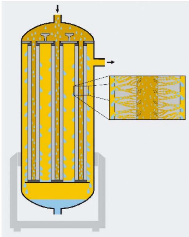
**Fig 3: Coalescence of water in diesel**
