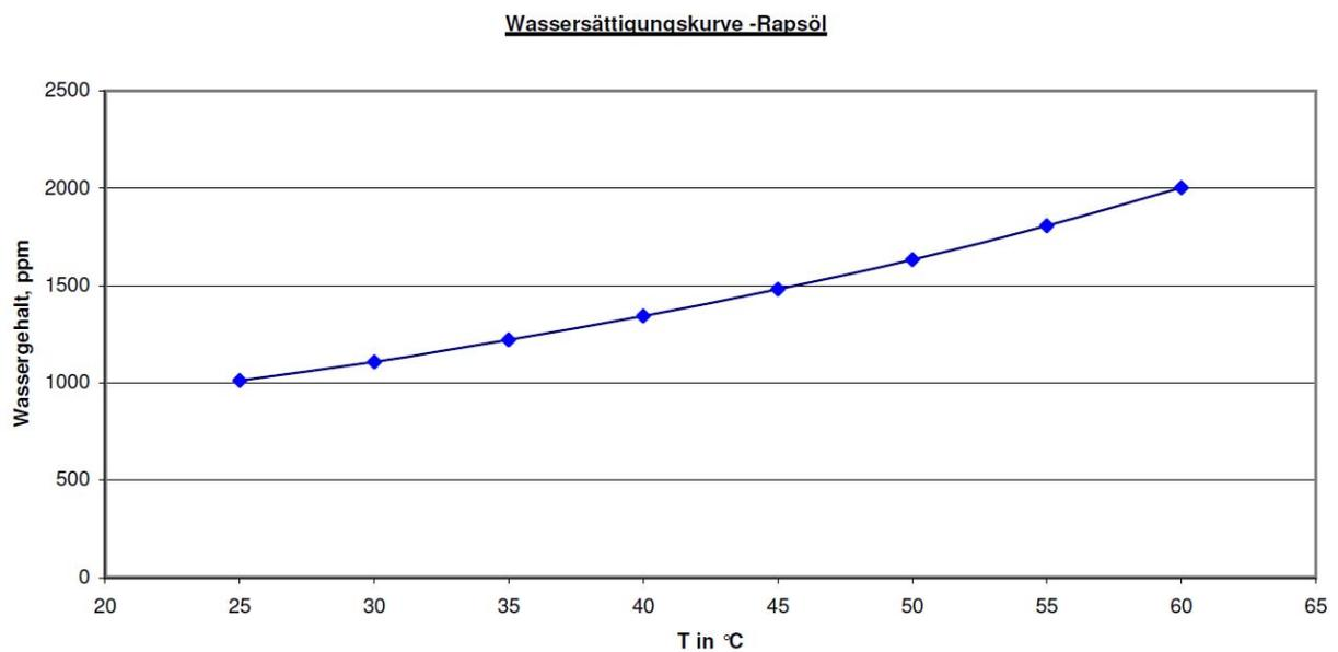
Figure 2: Water saturation curve for rapeseed oil (B100, France, 2013)
